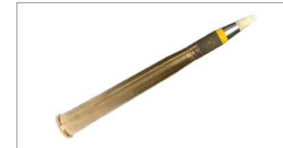
The projectile is mounted on a brass cartridge case which is filled with single base propellant multiperforated and fitted with a percussion primer.
